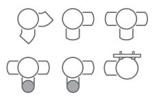
Available in the versions angle seat valve, angle valve, T-valve, cross valve, loopvalve, tank outlet valve
