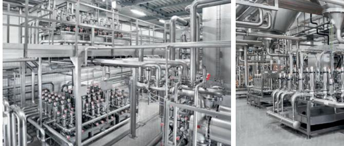
Two-level, fully-automatic valve manifolds with DN125/100 mixproof double seat valves, to connect ten tanks to seven filling lines.
