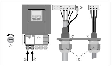
Figure 3-14: Electrical connection of the signal and field current cables, wall-mounted housing
