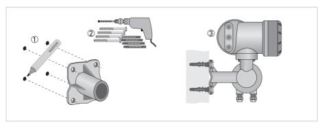
Figure 2-3: Wall mounting of the field housing
