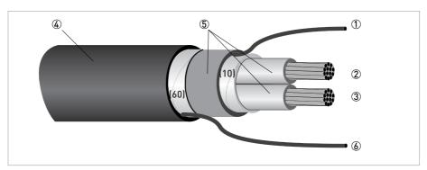
Figure 3-1: Construction of signal cable A
