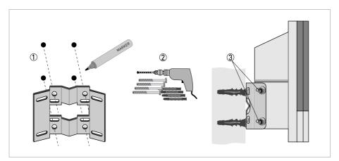
Figure 2-8: Wall mounting of the wall-mounted housing
