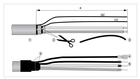
Figure 3-3: Signal cable A, preparation for wall-mounted housing
