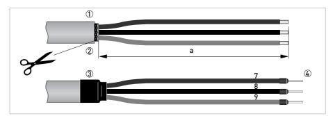
Figure 3-12: Field current cable C, preparation for the flow sensor  $% \left( 1\right) =\left( 1\right) \left( 1\right)$
