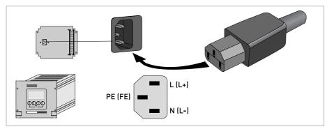
Figure 3-24: Power supply connection for 19" rack-mounted housing (28 TE)
