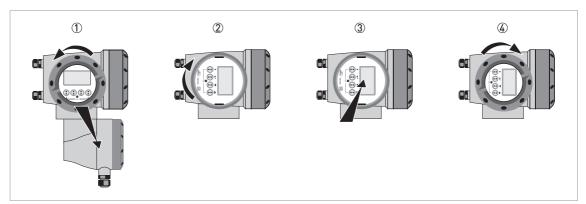
Figure 2-6: Turning the display of the field housing version
