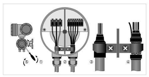
Figure 3-13: Electrical connection of the signal and field current cables, field housing
