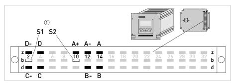
Figure 3-29: Terminal compartment for inputs and outputs in rack-mounted housing
