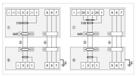
Figure 3-19: Connection diagram for flow sensor, field housing
