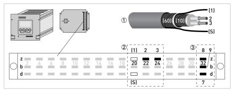
Figure 3-15: Connection signal cable A and field current cable
