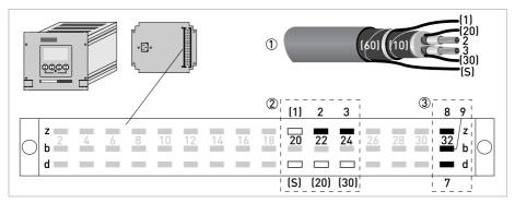
Figure 3-16: Connection signal cable B and field current cable
