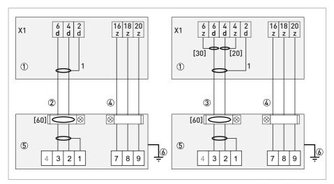
Figure 3-22: Connection diagram for flow sensor, 19" rack-mounted housing (21 TE)
