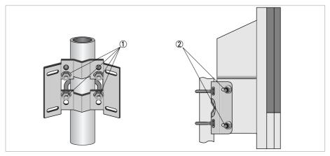
Figure 2-7: Pipe mounting of the wall-mounted housing
