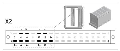
Figure 3-30: Terminal compartment for inputs and outputs in rack-mounted housing
