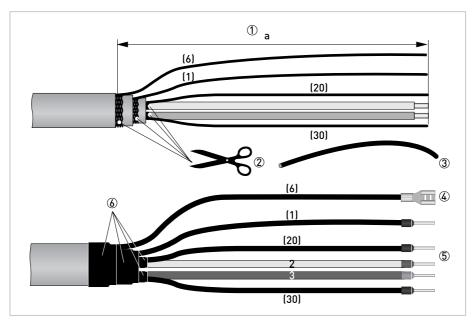
Figure 3-7: Signal cable B, preparation for wall-mounted housing
