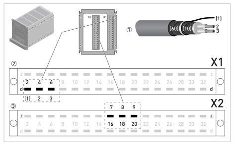
Figure 3-17: Connection signal cable A and field current cable
