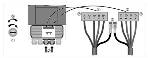
Figure 3-28: Connection of inputs and outputs in wall-mounted housing
