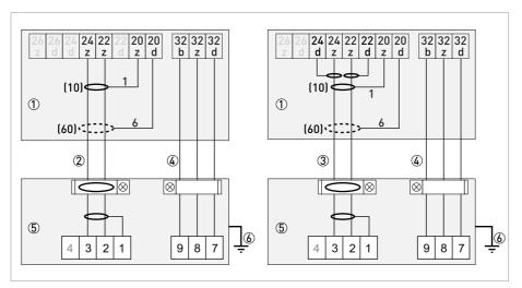
Figure 3-21: Connection diagram for flow sensor, 19" rack-mounted housing (28 TE)
