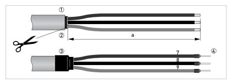
Figure 3-9: Field current cable C, preparation for the signal converter  $% \left( 1\right) =\left( 1\right) \left( 1\right) \left($
