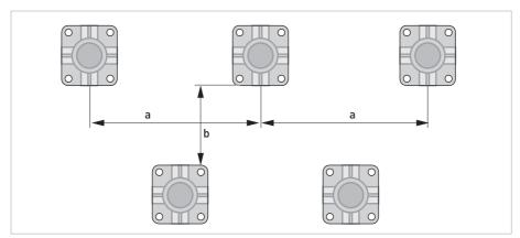
Figure 2-4: Mounting multiple devices next to each other
