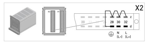
Figure 3-25: Power supply connection for 19" rack-mounted housing (21 TE)
