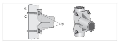
Figure 2-2: Pipe mounting of the field housing
