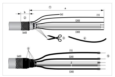
Figure 3-6: Signal cable B, preparation for field housing
