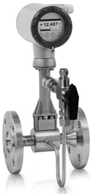
As an option, the **OPTISWIRL 4200** can be supplied with a shut-off valve to allow the pressure sensor to be exchanged without interrupting the process.
