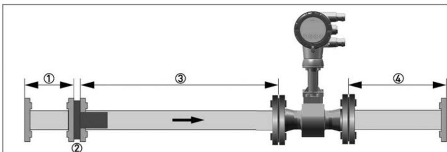
Figure 3-10: Flow straightener
