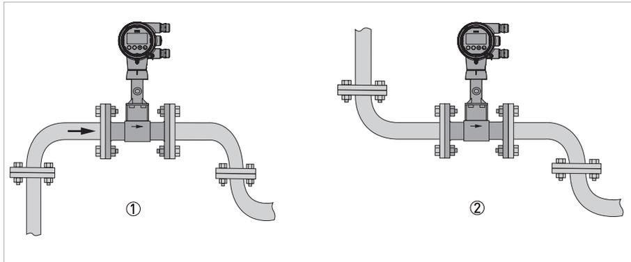
**Figure 3-3: Recommended installation**
