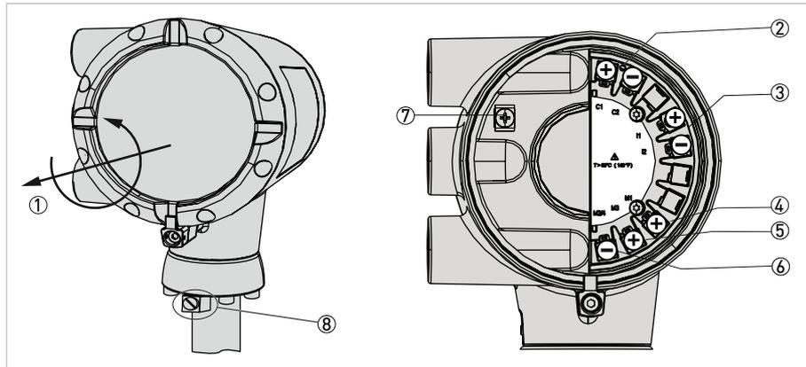
**Figure 4-1: Connecting the signal converter**
