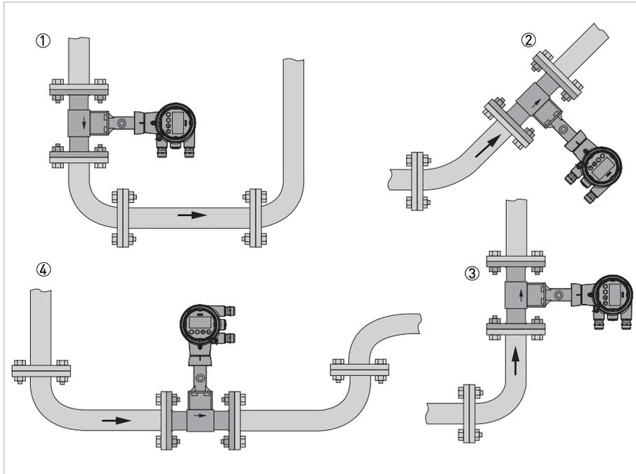
Figure 3-1: Recommended installation
