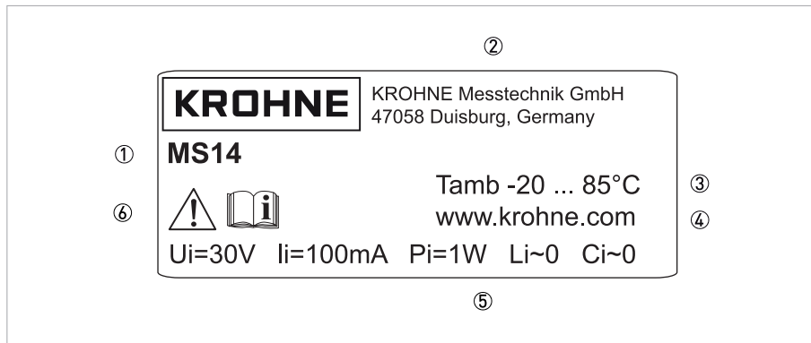
Figure 2-6: Marking of limit switches MS14
