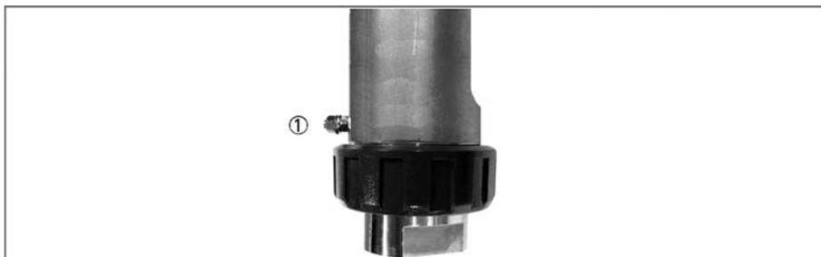
Figure 3-6: Ground terminal for VA40
