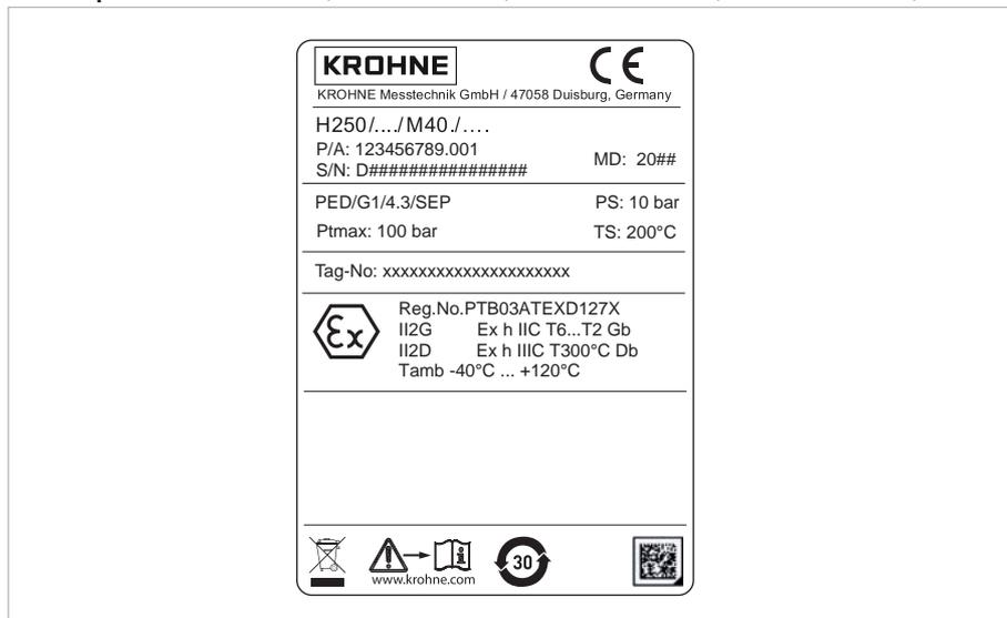
Figure 2-9: Example of a nameplate for H250 M40
