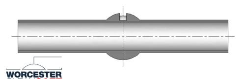
■ WK70 – CleanSafe has a bore equivalent to the tube so the media cannot settle (puddle) either side or within the valve and allows for self draining
