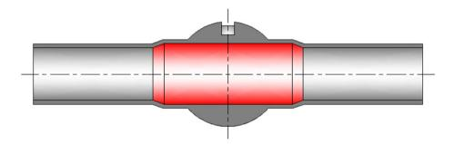
■ A59 – Full bore valve has a larger bore than the tube and therefore media would collect (puddle) within the valve
