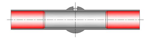
■ A44 – Reduced bore valve has a smaller bore than the tube and therefore media would collect (puddle) either side of the valve
