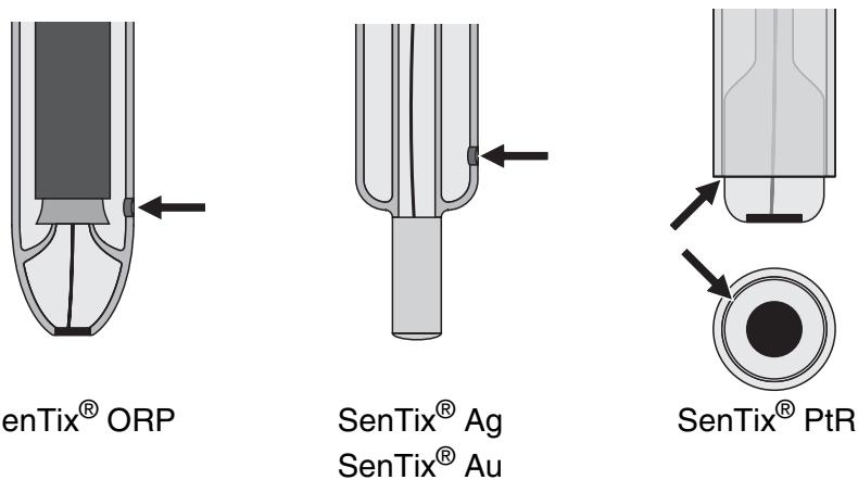
At the same time the level of the reference electrolyte in SenTix® ORP, SenTix® Au and SenTix® Ag electrodes must be at least 2 cm above the level of the solution.
