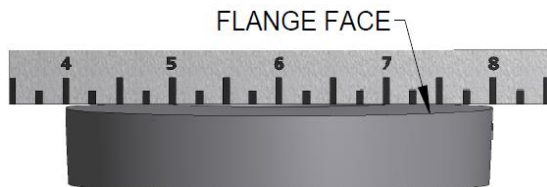
Figure 3 - Measuring for Flatness
