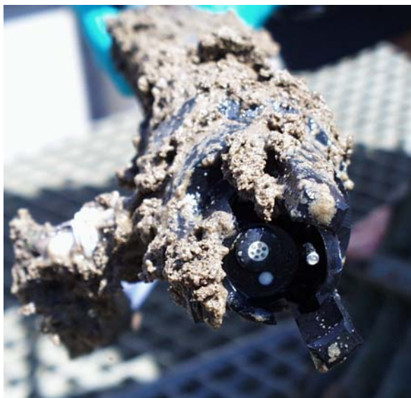
Fig. 16 Left: CH cleaning head to screw on the VARiON ®Plus 700 IQ Right: Successfully keeping free the measurement electrodes during operation
