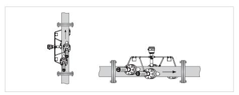
Figure 2-11: Horizontal or vertical installation
