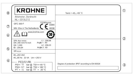
Figure 2-4: Example of nameplate
