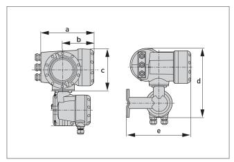
Figure 4-2: Field housing (F) - remote version.
