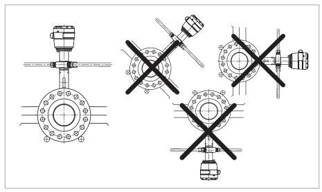
Figure 2-12: Mounting position
