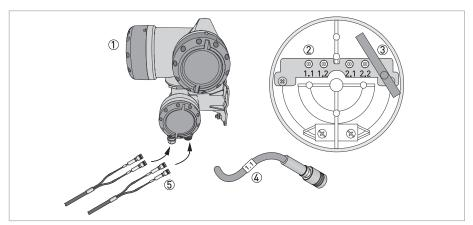
Figure 3-1: Connection of signal cable to signal converter
