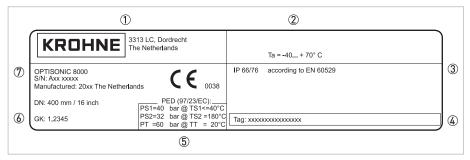
Figure 2-3: Example of nameplate
