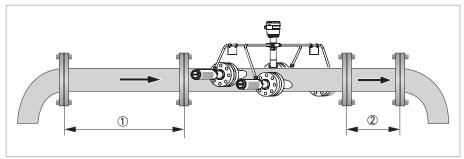
Figure 2-8: Recommended inlet and outlet
