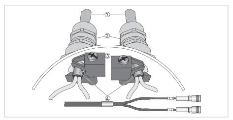
Figure 3-2: Clamp the cables on the shielding bush
