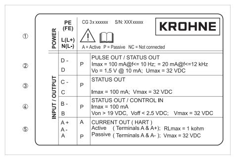
Figure 2-5: Example of a nameplate for electrical connection data of inputs and outputs
