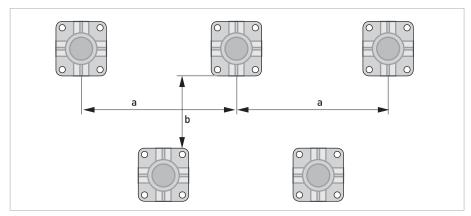
Figure 2-15: Mounting multiple devices next to each other
