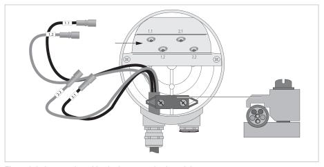
Figure 3-3: Connect the cables in the connection box of the sensor  $% \left( 1\right) =\left( 1\right) \left( 1\right)$
