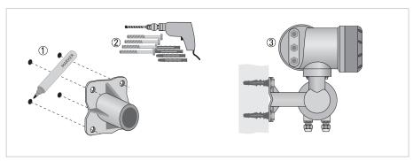
Figure 2-14: Wall mounting of the field housing
