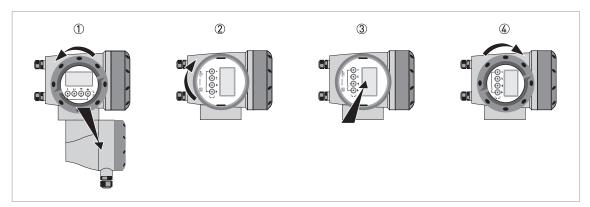
Figure 2-16: Turning the display of the field housing version
