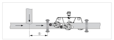
Figure 2-9: Distance behind a T-section
