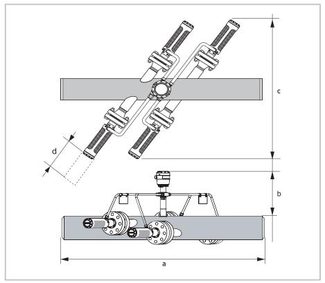
Figure 4-1: Top and front view of the OPTISONIC 8000
