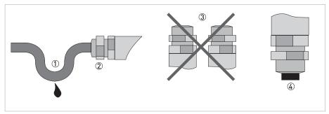
Figure 3-5: Protect housing from dust and water
