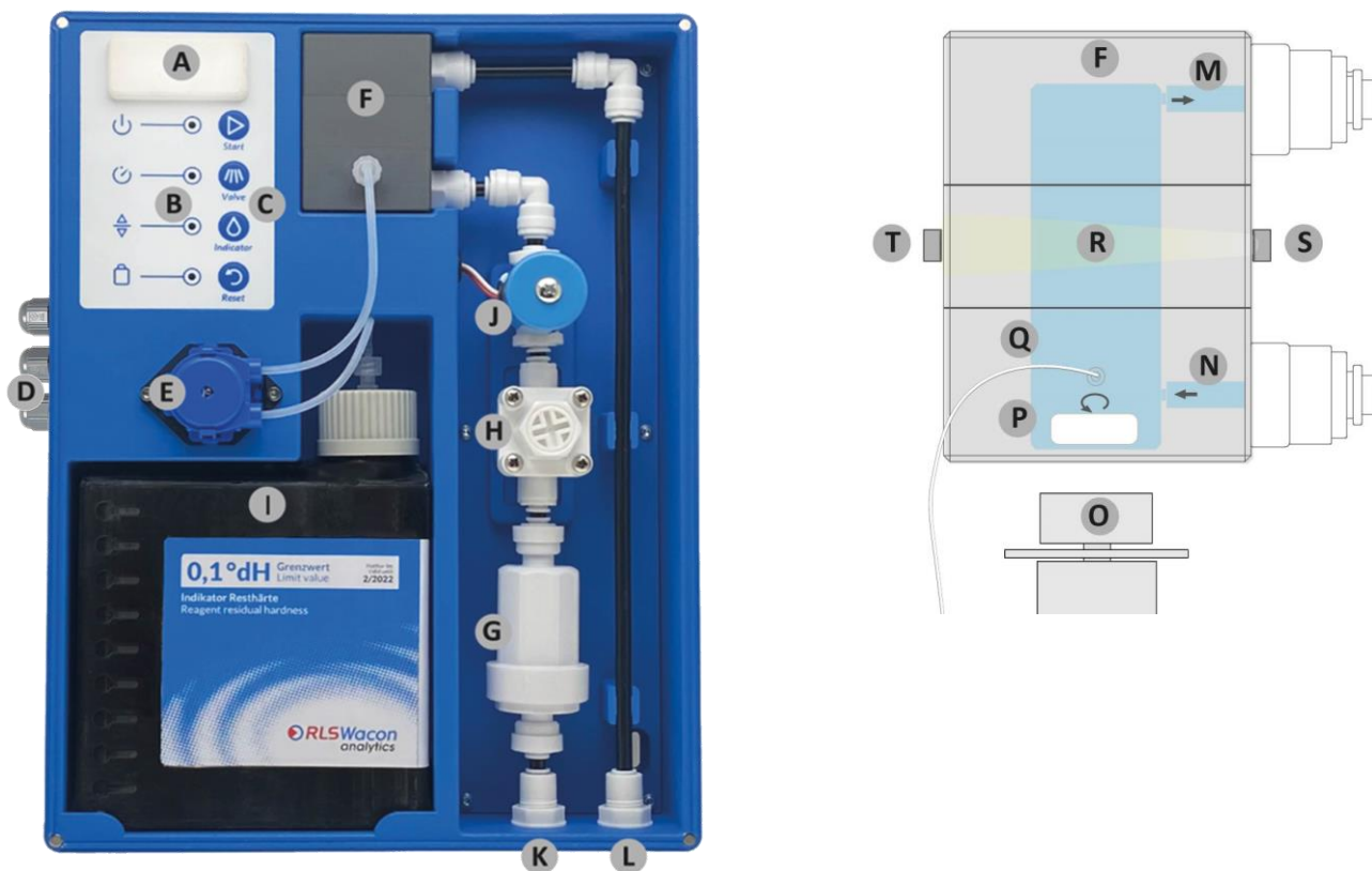
Illustration 4: LIMES analyzer with indicator bottle installed (I.), schematic representation of the measuring chamber (r.)
