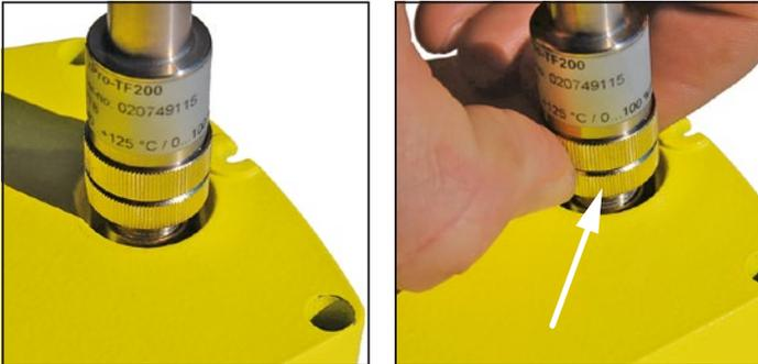
For mounting the sensor must be plugged into the socket and screwed on the sensor by turning the lower knurled screw clockwise. Tighten hand-screwed only. A small clearance between transmitter and sensor has to be accepted due to production conditions.
