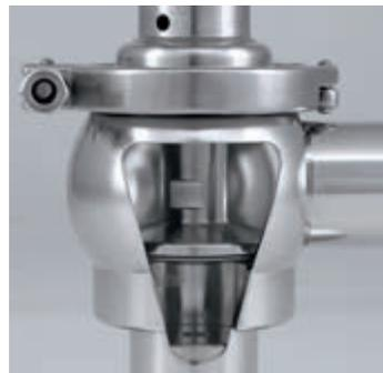
**Precise to the full stroke:** Our overflow valves relieve pressurised spaces when impermissible pressures arise. The medium is routed to the exterior or into a closed system in a controlled manner. The flow-optimised disc geometry ensures precise opening and closing behaviour as well as high flow capacity.
