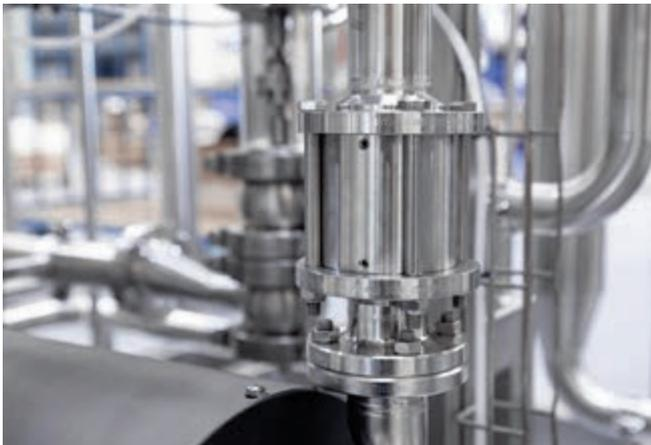
They open autonomously, as soon as the inlet-side dynamic pressure exceeds the spring force and close automatically with a corresponding pressure drop or flow in the opposite direction. This means for example that the suction line will not run dry after switching off the pump. In the depressurised condition the valve disc is pushed against the seat seal by the spring preload.
