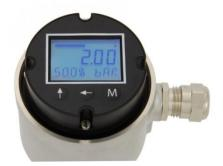
Unscrew the cover to get access to the push buttons of the display. The display can be turned max. 180° to put it in the desired position for reading. The complete display unit can be taken out to be able to adjust the transmitter. Be careful when taking out the display as the length of the wiring is limited. Please ensure that the cover is fastened properly after adjusting the display to ensure the sealing of the housing.
