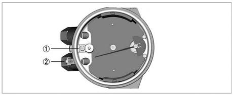
Figure 3-2: Ground terminal for H250/M40.
