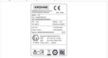
Figure 2-8: Example of a nameplate for DK32 HT
