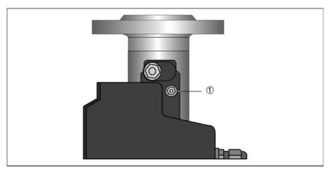
Figure 3-4: Ground terminal for H250/M8MG/.
