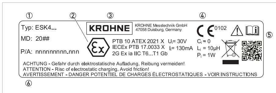
Figure 2-2: Example of a nameplate for a standard version
