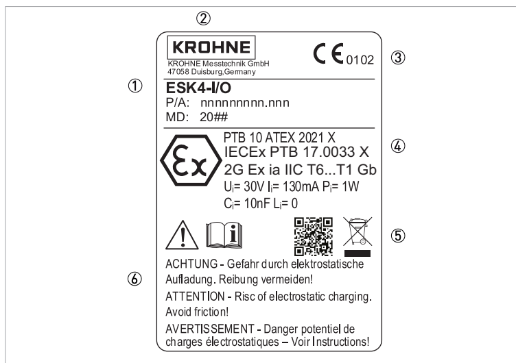
Figure 2-4: Example of nameplate for a version with I/O
