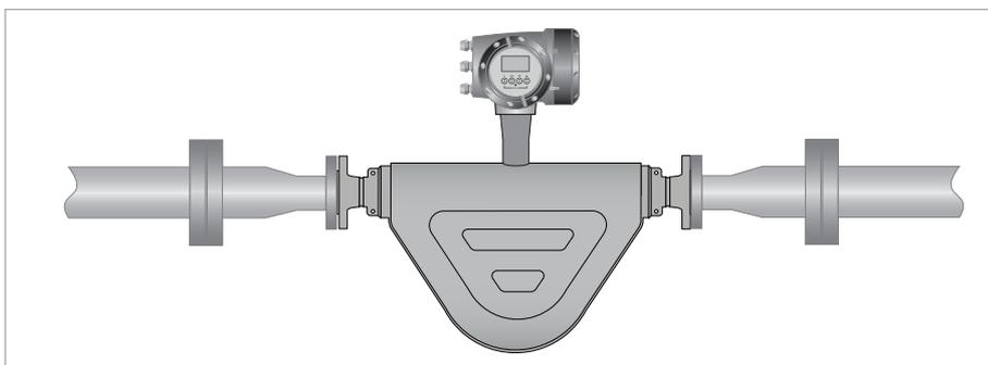
Always avoid extreme step changes in pipe size. Use pipework reducers, where there is a large difference between pipework size and meter flanges.
