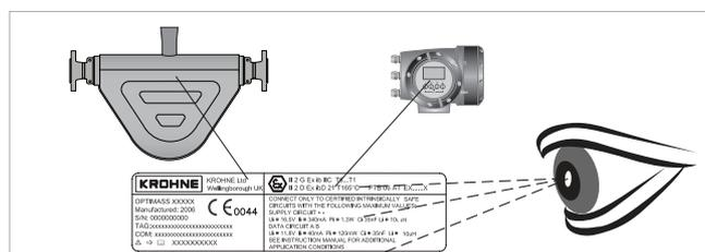
To ensure the PED integrity of the meter, you **MUST** check that the serial numbers on the converter nameplate and the sensor nameplate are the same.
