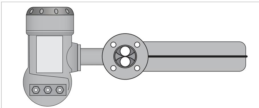
The meter can be installed with the converter (or remote junction box) on the side of the meter so that the measuring tubes are sitting one above the other. Avoid this method of installation where there is a two phase process flow, or where the process fluid contains gas. If this situation cannot be avoided, please contact the manufacturer for advice.
