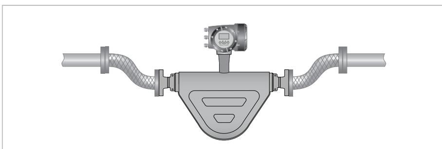
Flexible connections can be used but because of the high flow rates associated with large diameter meters, it is recommended that flexible connections are not used on meters larger than size 80.
