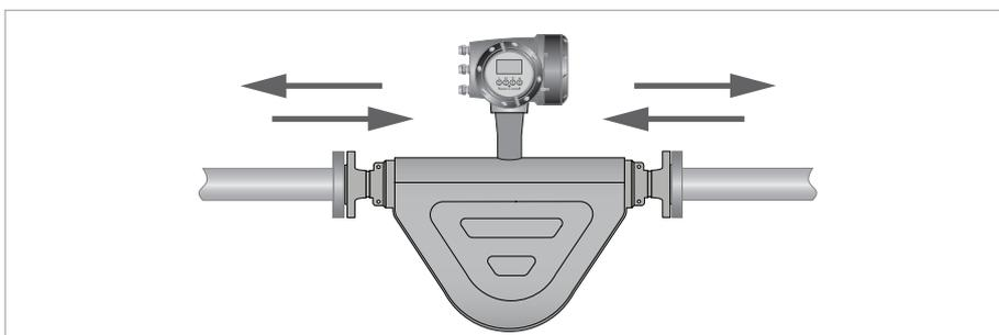
Mass flowmeters have a maximum level of force (negative or positive) that can be applied to the ends of the meter. Refer to the table below for permitted forces.
