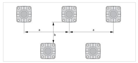
Figure 3-17: Mounting multiple devices next to each other
