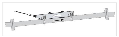
Figure 3-2: Install on a slightly ascending pipe section
