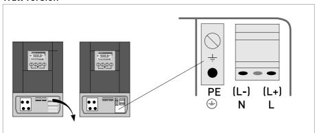
Figure 4-6: Signal converter wall version, power supply
