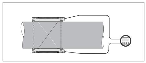
Figure 3-11: X beam configuration of medium version
