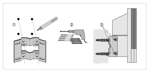
Figure 3-18: Wall mounting of the wall-mounted housing
