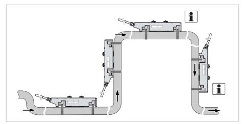
Figure 3-4: Installation in bending pipes (90°)
