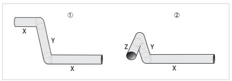
Figure 3-3: 2 and/or 3 dimensional bends upstream of the flowmeter
