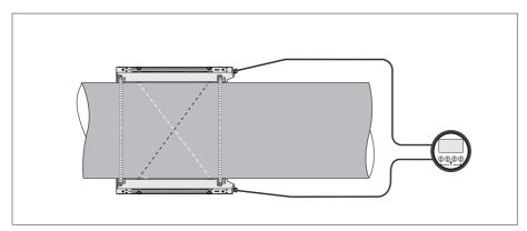
Figure 1-6: X beam configuration of medium version
