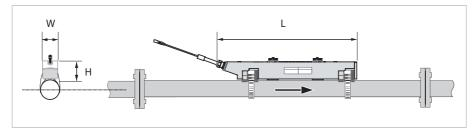
Figure 2-2: Dimensions clamp-on sensor rail(s)
