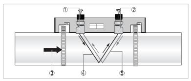
Figure 1-8: Measuring principle (example reflected path set-up)
