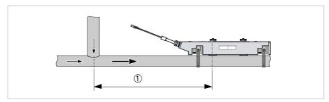
Figure 3-6: Distance behind a T-section
