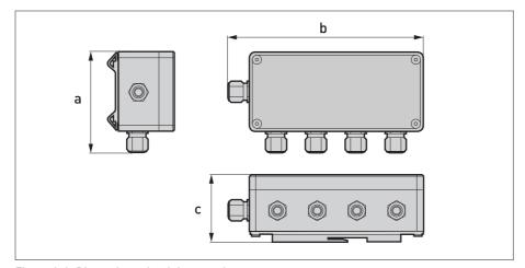
Figure 2-3: Dimensions aluminium version
