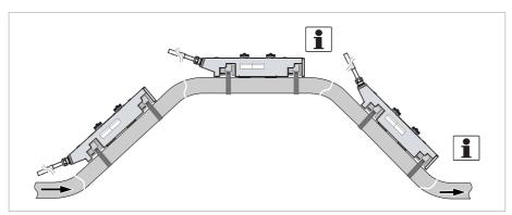
Figure 3-5: Installation in bending pipes (45°)
