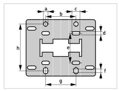
Figure 2-6: Dimensions of mounting plate of wall-mounted housing
