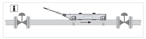
Figure 3-9: Position of control valve
