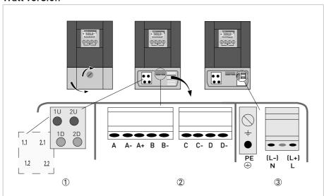
Figure 4-3: Construction of wall version
