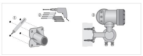
Figure 3-16: Wall mounting of the field housing
