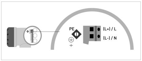
Figure 4-5: Signal converter field version, power supply connections
