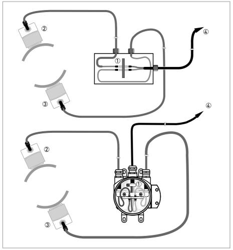
Figure 4-12: Example of large sensor rail connections with cable (splitter) box
