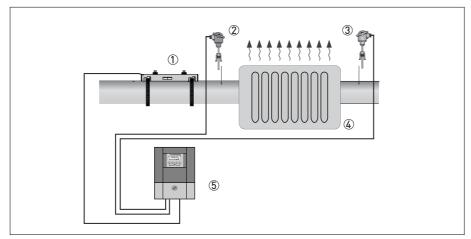
Figure 3-12: Energy measurement of heat/cold producer/consumer
