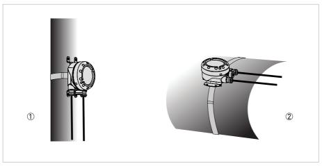
Figure 3-14: Pipe (pole) mounting or installation on the pipe line
