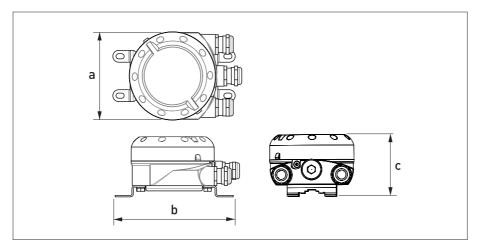
Figure 2-4: Dimensions stainless steel version
