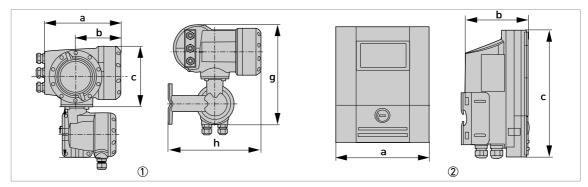
Figure 2-1: Dimensions of housing
