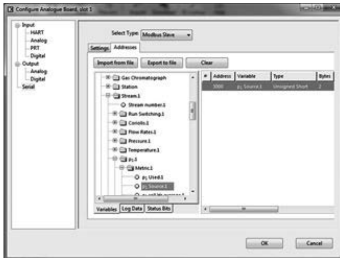
Figure 57 Density serial input selection
