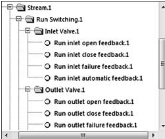
Figure 130 Run switching digital input selection
