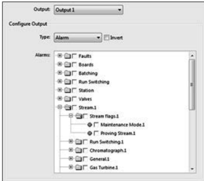
Figure 35 Configure alarm output
