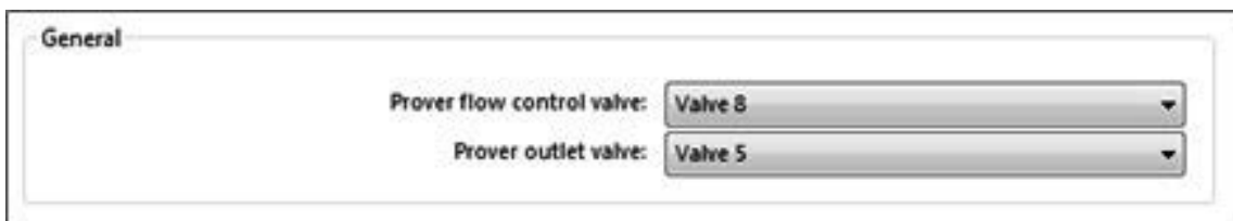
Figure 154 Prover valve control, uni-directional or small volume
