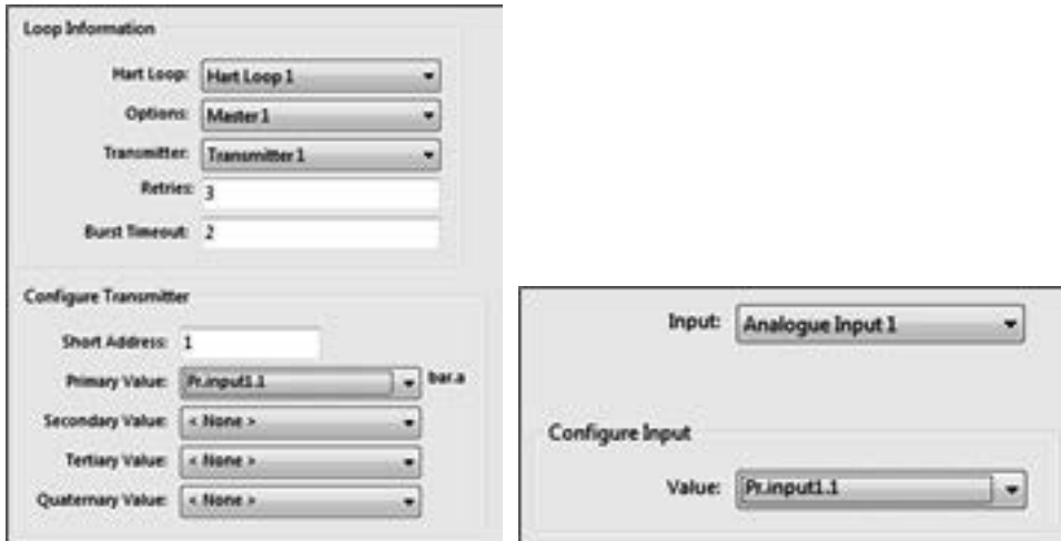
Figure 53 Pressure input selection
