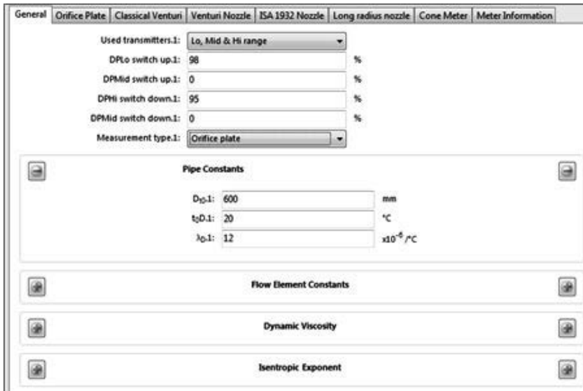
Figure 73 Differential pressure General section
