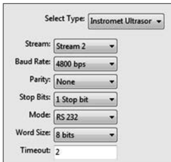
Figure 42 Setup of an Instromet ultrasonic meter in Hardware selection
