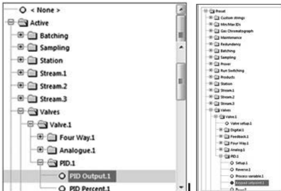
Figure 166 Select the PID valve ID and the Preset keypad setpoint ID
