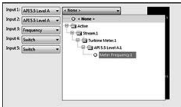
Figure 40 Setup of a Level A dual pulse in Hardware selection
