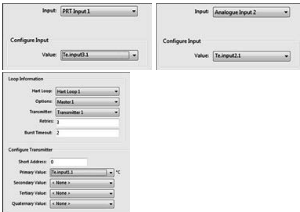
Figure 50 Temperature input selection
