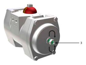
D. With the help of suitable size Allen (hex.) key, rotate the stop bolt (3) clockwise to increase (counter-clockwise to decrease) the angular stoke
