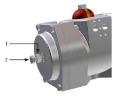
E. Hold the stop bolt (2) with a spanner and carefully tighten the stop nut (1)
