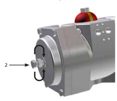
C. With the help of a suitable spanner, rotate the stop bolt (2) clockwise to increase (counter-clockwise to decrease) the angular stoke
