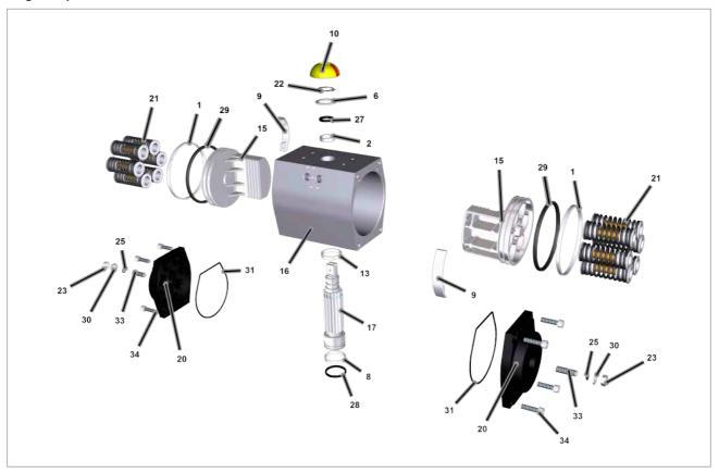
Fig 17.1 Single Stop GT Actuator
