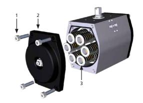
10. With an Allen (hex.) key remove the 4 screws (1) from the other end cap (2)
